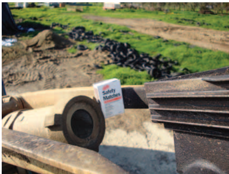
The large orifice of the hard hose irrigator minimises blockages.
