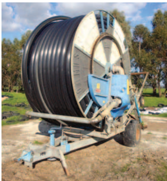
The Ocmis hard hose irrigator used to apply effluent.
